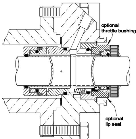
Optional floating throttle bushing or lip seal design for frame 1 ANSI stuffing box with .312 packing space. Provides solution for dissolved and undissolved solids and thermally sensitive fluid applications.
