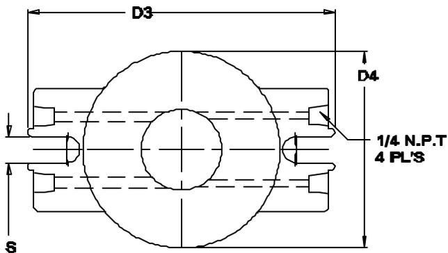
Quench & Drain optional on this seal model.
