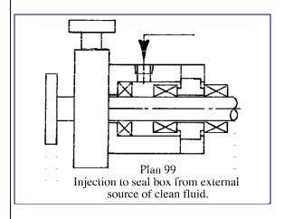
The stuffing box/seal chamber. is flushed from a clean, cool external source at a rate and temperature to maintain a proper environment for the seal. The flush must be sufficient to prevent the pumped fluid from entering the seal chamber. A close clearance bushing installed in the bottom of the seal chamber will reduce the flush required by increasing the velocity at the throat at a given flow.
