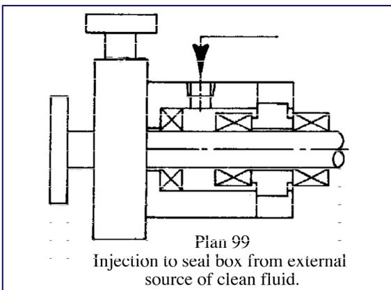
The stuffing box/seal chamber is flushed from a clean, cool external source at a rate and temperature to maintain a proper environment for the seal. The flush must be sufficient to prevent the pumped fluid from entering the seal chamber. A close clearance bushing installed in the bottom of the seal chamber will reduce the flush required by increasing the velocity at the throat at a given flow.
