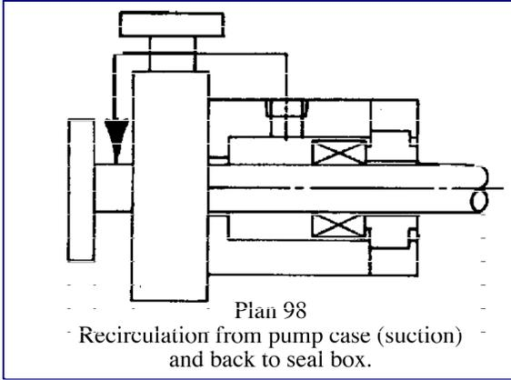
A line is connected from the pump suction to the stuffing box/seal chamber. This is used to reduce pressure in the seal chamber enabling the seal to run cooler and to recirculate liquid and solids away from the seal faces.
